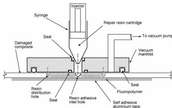
**Figure 6 - Resin Infusion or Injection Repair**
