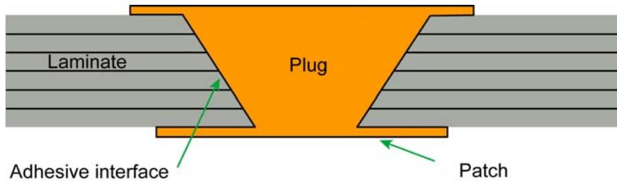
**Figure 5 - Adhesive Bonded Plug Repair**
