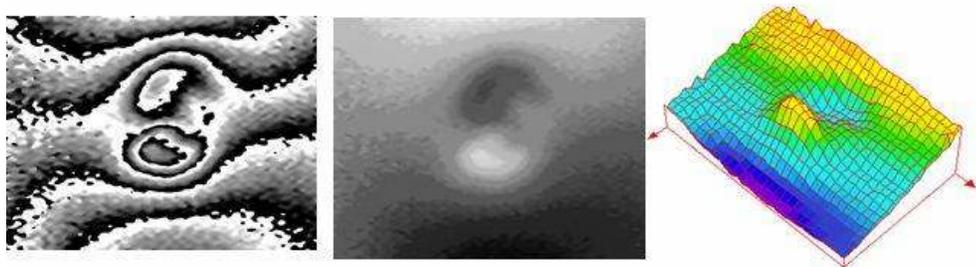
**Fig.2.14. Phase stepped fringe pattern, unwrapped image and 3D processed images of impact damage in an aerospace panel.**
