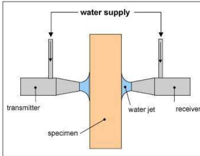
**Fig.2.5. Immersion through-transmission test set-up implemented with jet probes**
