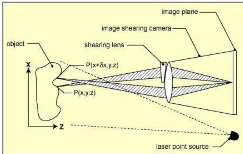
**Fig.2.13. Basic Set-up for conventional shearography**
