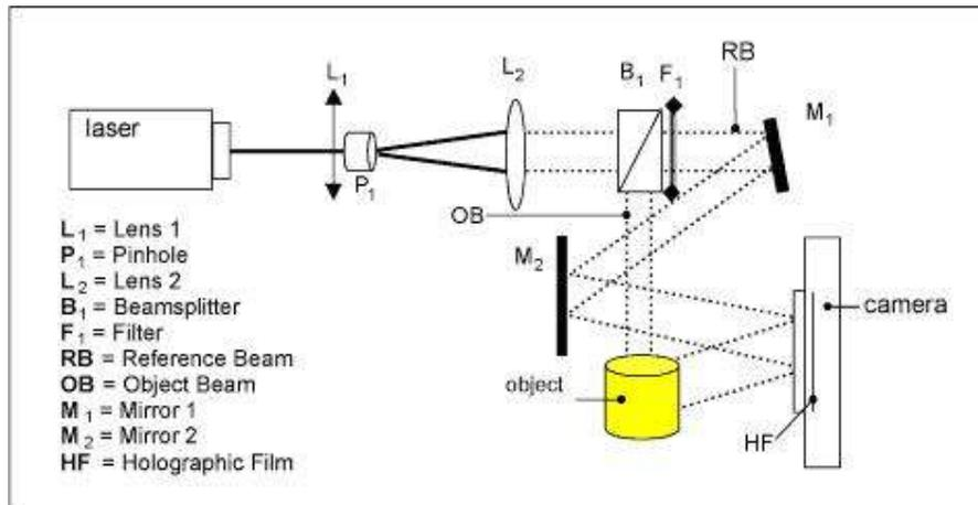
Fig.2.9. Optical holography set-up
