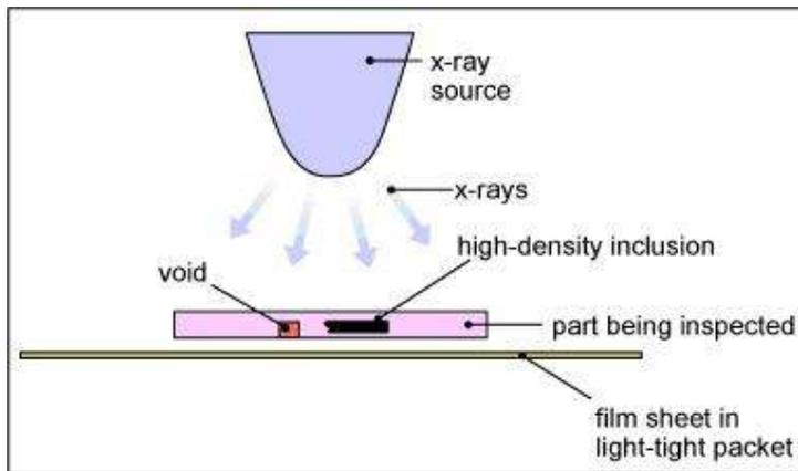
**Fig.2.12. Schematic set-up of X-ray radiography test**
