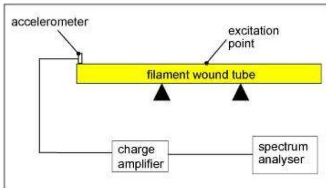
**Fig.2.8. Schematic diagram of apparatus for checking modal frequencies of filament wound CFRP tubes**
