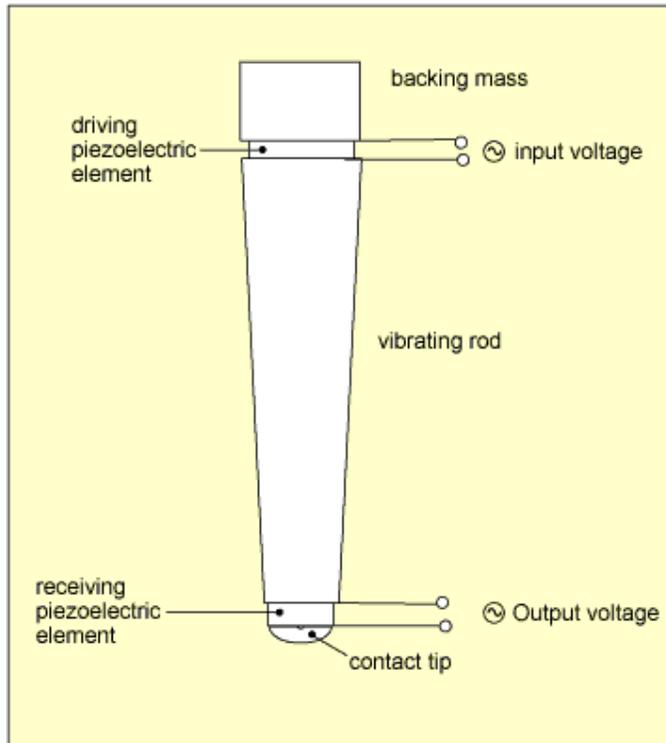
**Fig.2.11. Probe for mechanical impedance method**
