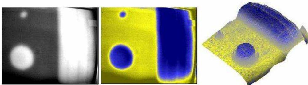
**Figure 2.18. Black and white, colour enhanced and 3D images of artificial delaminations in wind turbine blade.**
