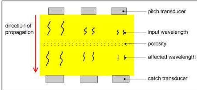
**Fig.2.6. Wavelength interaction illustration for ultrasonic spectroscopy**
