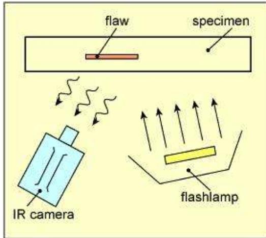
**Fig.2.17. Experimental set-up for thermal pulse thermography**
