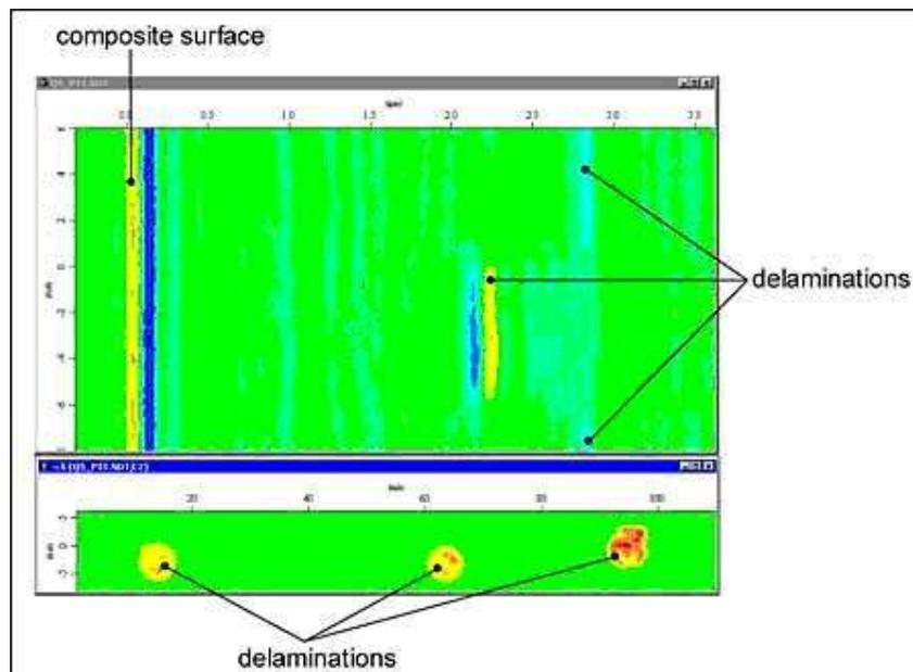
**Fig.2.3. Ultrasonic image of delamination in carbon fibre composite (B and C-scans)**
