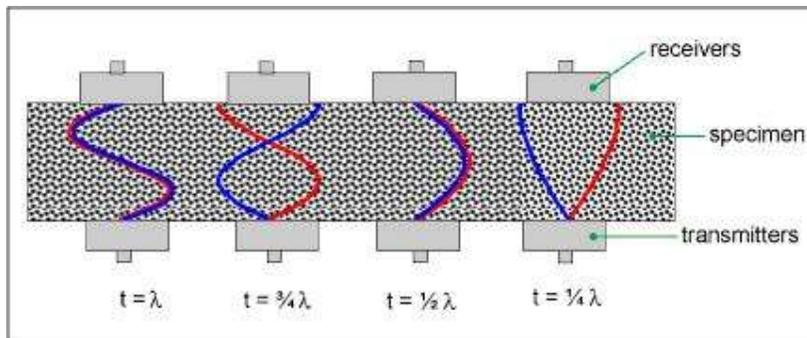
**Fig.2.7. Interference effects in thin specimens tested by ultrasonic spectroscopy (through-transmission configuration shown). Two phases of received signal shown by red and blue lines**
