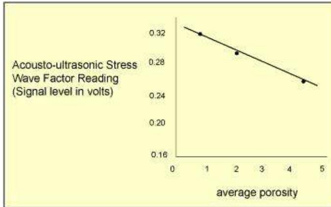
**Fig.2.16. Acousto-ultrasonic detection of porosity**
