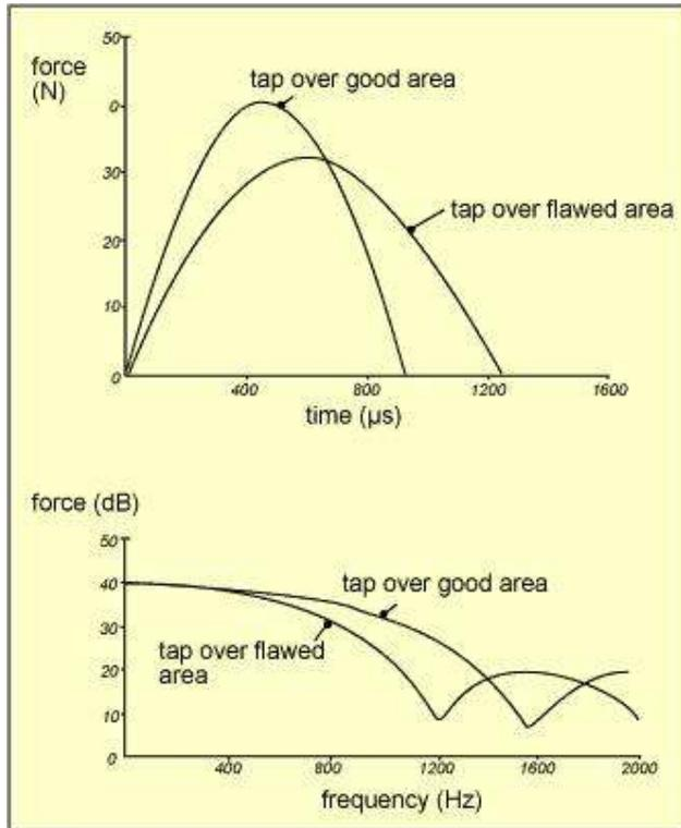
**Fig.2.10. Interacting force in hammer tip produced by the coin-tap test applied over composite**
