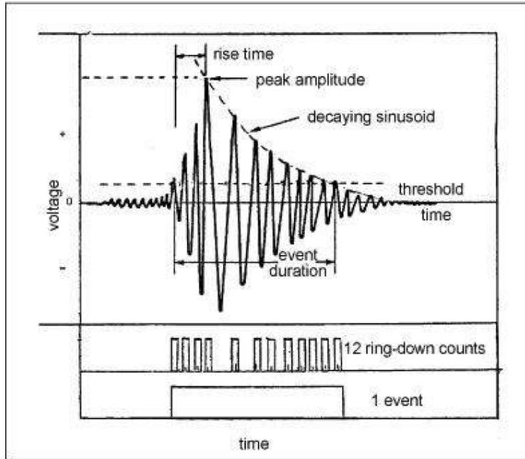
**Fig.2.15. Amplified signal from a piezoelectric transducer illustrating 'ring-down' and event counting**
