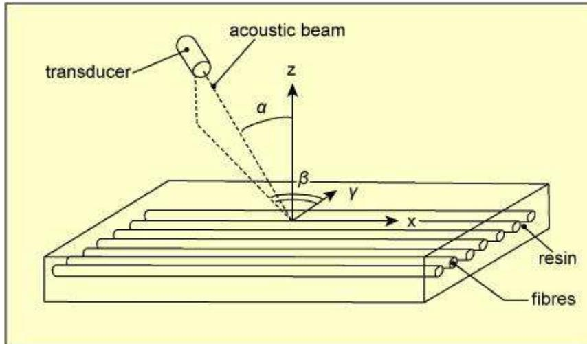
**Fig.2.4. The back-scatter technique**
