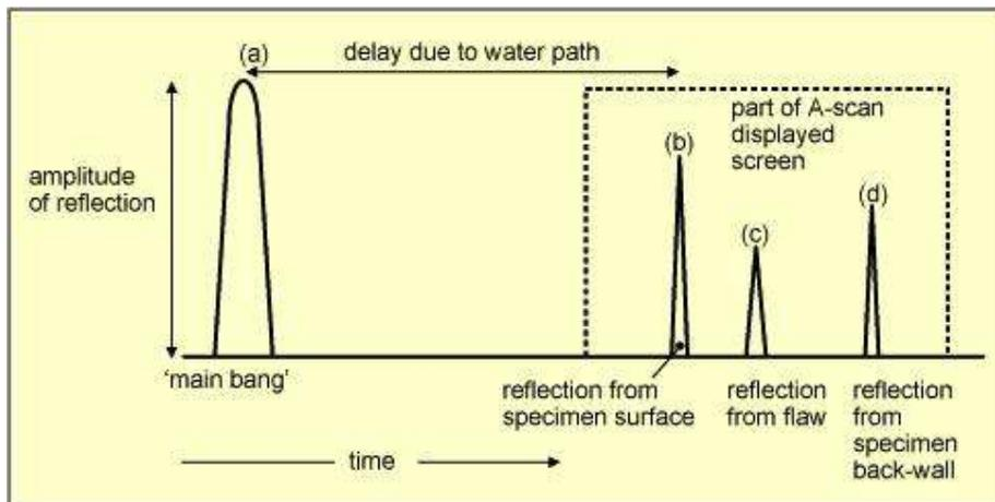
**Fig.2.2. Diagrammatic A-scan display for a typical pulse-echo immersion test**
