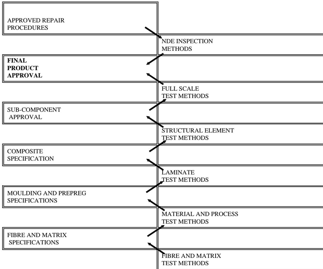
**Figure 1. Chain of validation for composites products**
