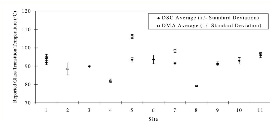
**Figure 3. DSC and DMA results on unreinforced polyester [13]**
