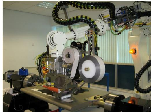
Automated Dynamics fibre placement machine at AMRC with Boeing Composites Centre (courtesy of AMRC with Boeing Composites Centre)
