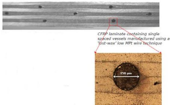
Vessels created within a composites to facilitate self-curing (Courtesy of the University of Bristol)
